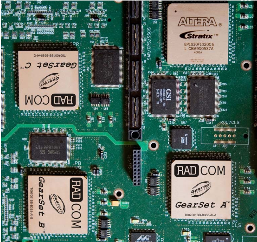
Implementation of the GearSet: Detail from the main board of RADCOM's new, high performance R70 probe
